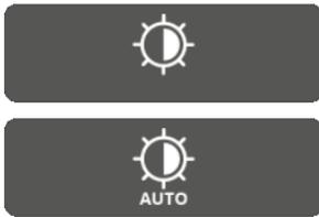
The brightness is by default set to automatic so the image is optimizing the brightness with respect to the signal it obtains. This setting can be switched to locked, after which the brightness will stay fixed. The locked state could be used for comparison applications, in case all other image parameters are fixed.
