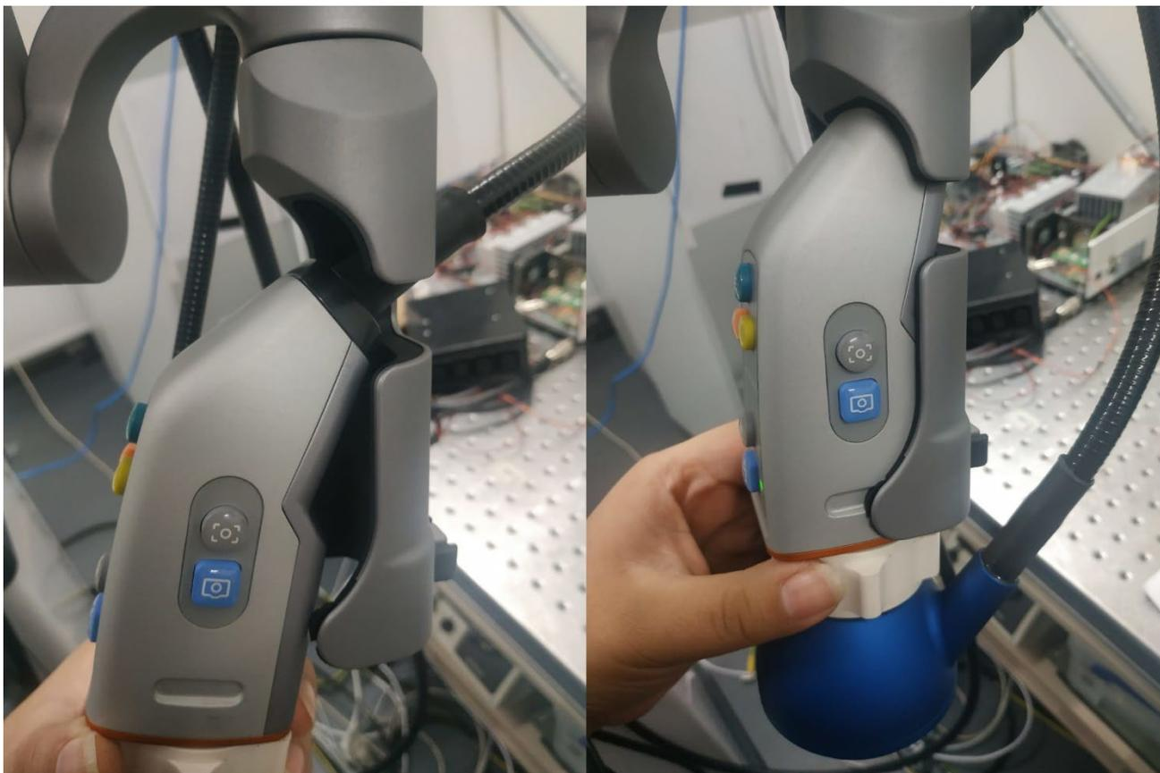
Figure 14: Camera positioned in arm gripper
