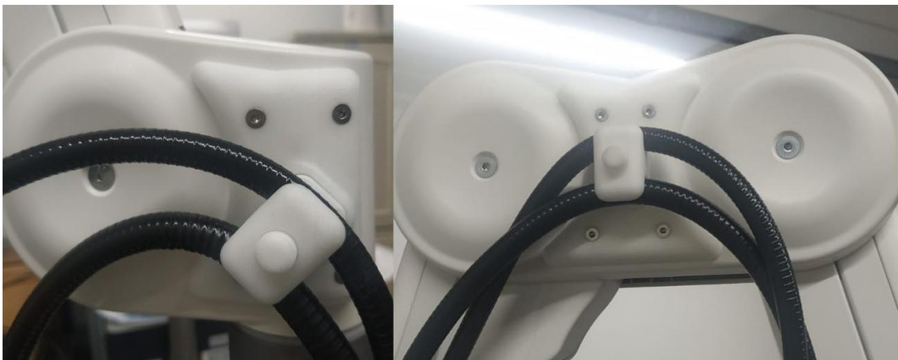
Figure 15: Cables secured in camera arm
