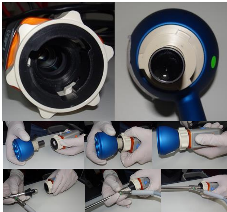
Figure 4: Connecting the ring light/Laparoscope to the camera
