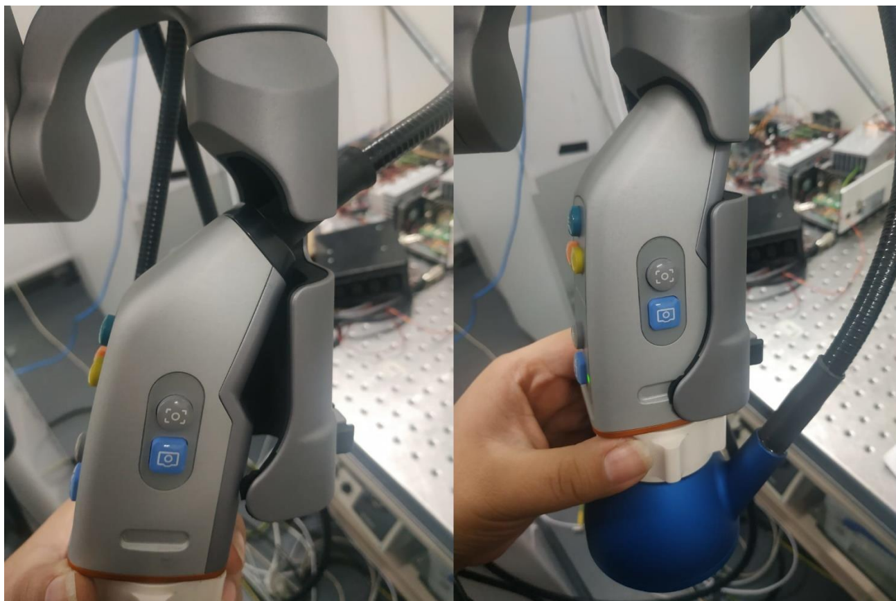
Figure 14: Camera positioned in arm gripper
