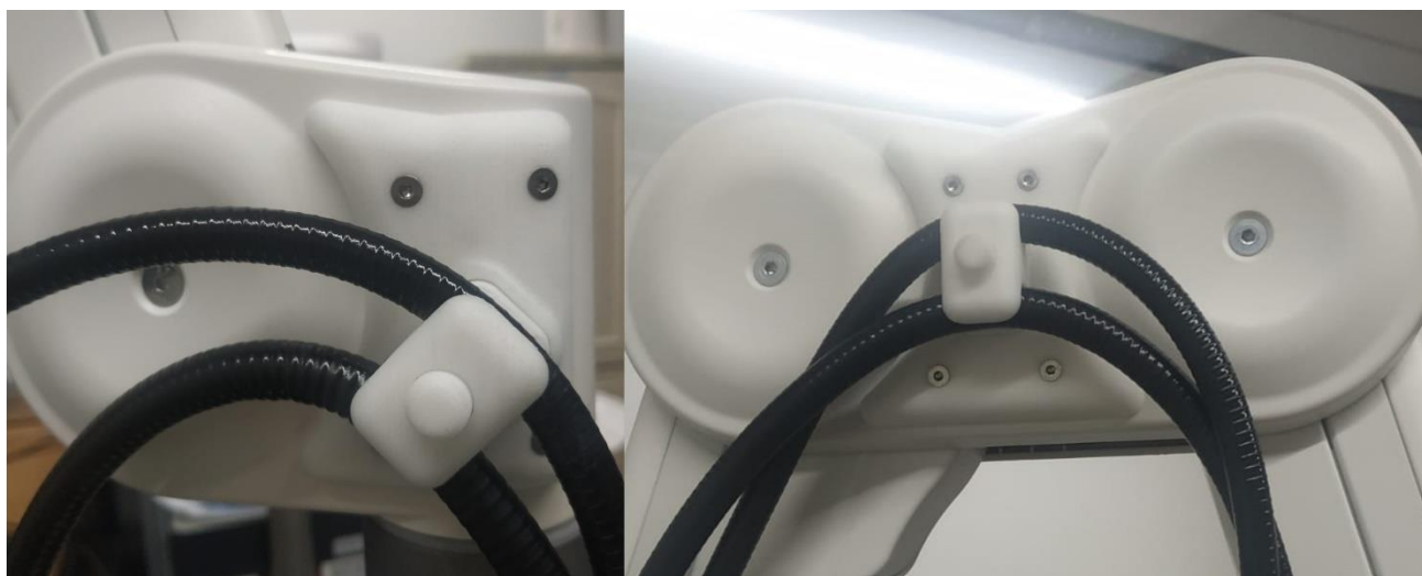
Figure 15: Cables secured in camera arm
