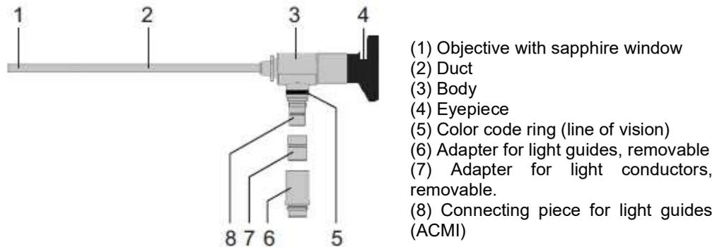
Figure 1: Construction of the Laparoscope
